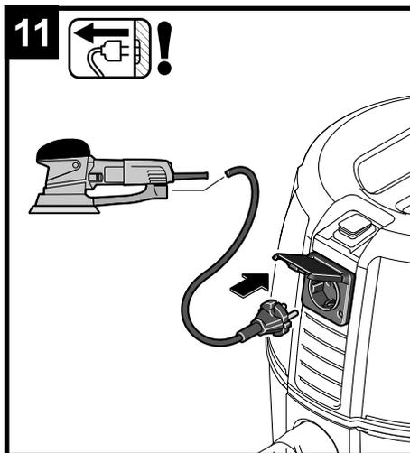
Only Choosing "AUTO" button vacuum cleaner works while the electric tool does; vacuum cleaner stops working after electric tool is closed. Only choosing "I" button, vacuum cleaner works yet the electric tool doesn't work When the "AUTO" button and "I" button is in the same level, both the vacuum cleaner and electric tool don't work for the electricity is cut off.
